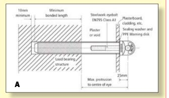
We also offer **Cantilever Anchor Devices** for use in dry lined walls or in conjunction with plasterboard, cladding etc. Where the distance from the face of the load bearing structure to the collar of the eyebolt does not exceed 25mm, a **spacer sleeve** may be placed under the eyebolt collar to provide the necessary support (Fig. A).
