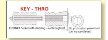
KEY-THRO Standard KEYANKA socket with additional M12 threaded extender. For use as through bolt fixing (e.g. in cavity walls). NO cantilever permitted.
