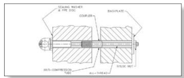
Eyebolt extended with threaded connector and all-thread for use as a through-bolt in solid or cavity wall. (BS 7883 Fig. 9)
