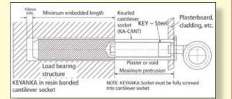
**KEY-CANT** Knurled cantilever socket for use in conjunction with standard **KEY-STEEL KEYANKA** socket in concrete and masonry.
