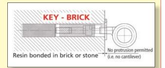
KEY-BRICK Standard KEYANKA socket with knurled extension suitable for resin bonding into min. 225mm thick solid masonry. NO cantilever permitted.
