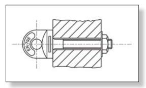
75mm shank length used ONLY on steel structures (BS 7883 Fig 9)
